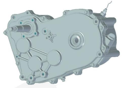
3. Remove the bolts on the shift cover and remove the shift cover. Remove shift cam, shift limit spring, and shift shaft, etc.
