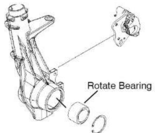
7. Rotate hub. It should rotate smoothly without binding or rough spots or side play.
