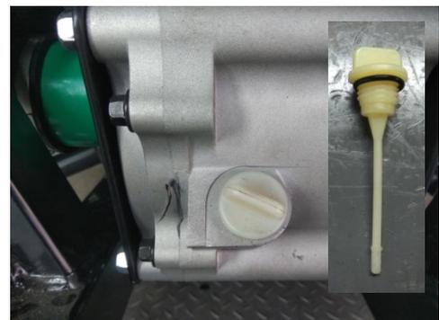
4. Check the O-ring for damage and replace it if necessary.
