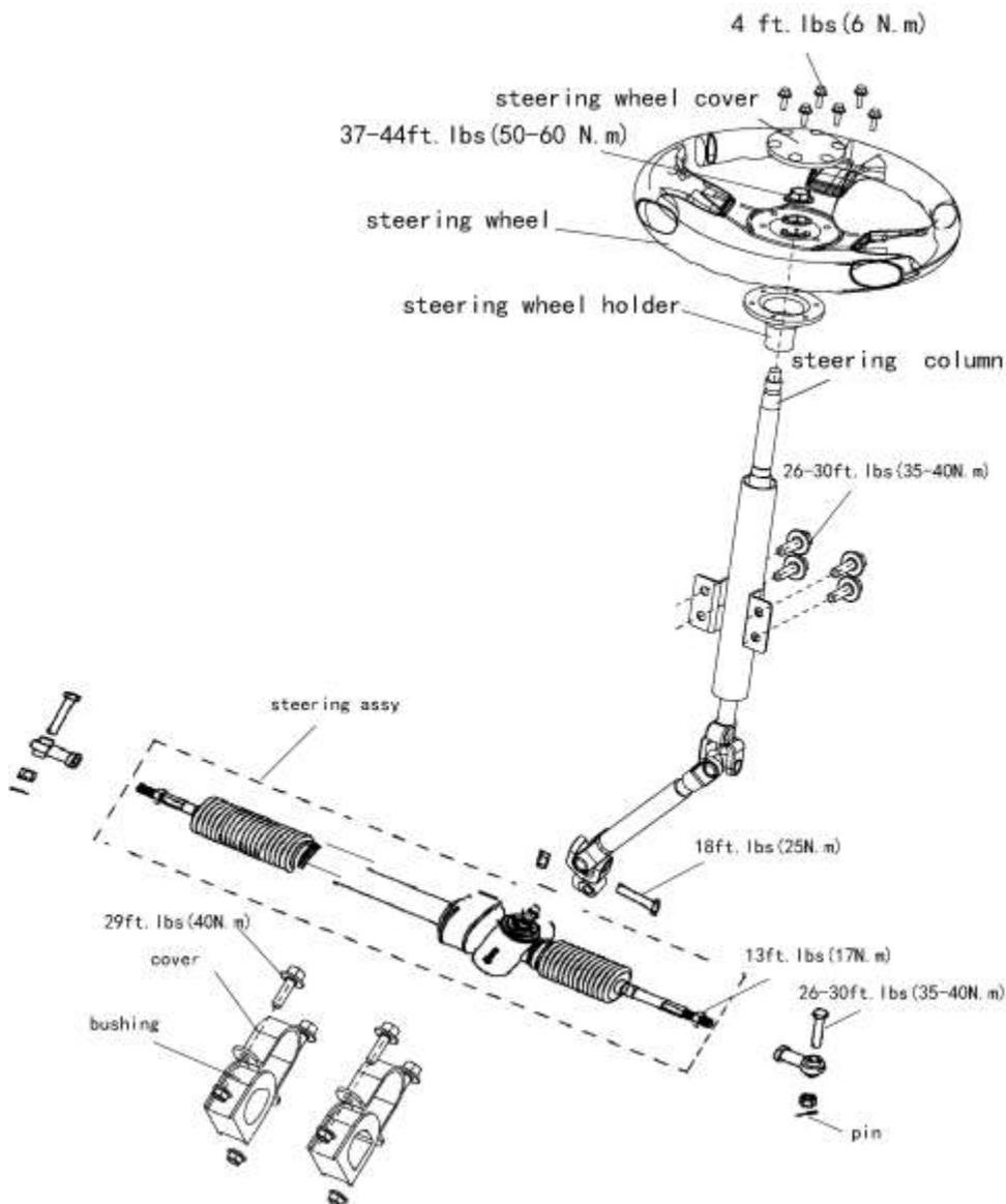
1. With the steering wheel cover bolts removed, remove the steering wheel cover and the steering wheel.
