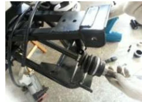
5. Loosen two bolts that secure the rear knuckle to the A-arm. Remove the rear knuckle assembly by sliding it off of the axle.
