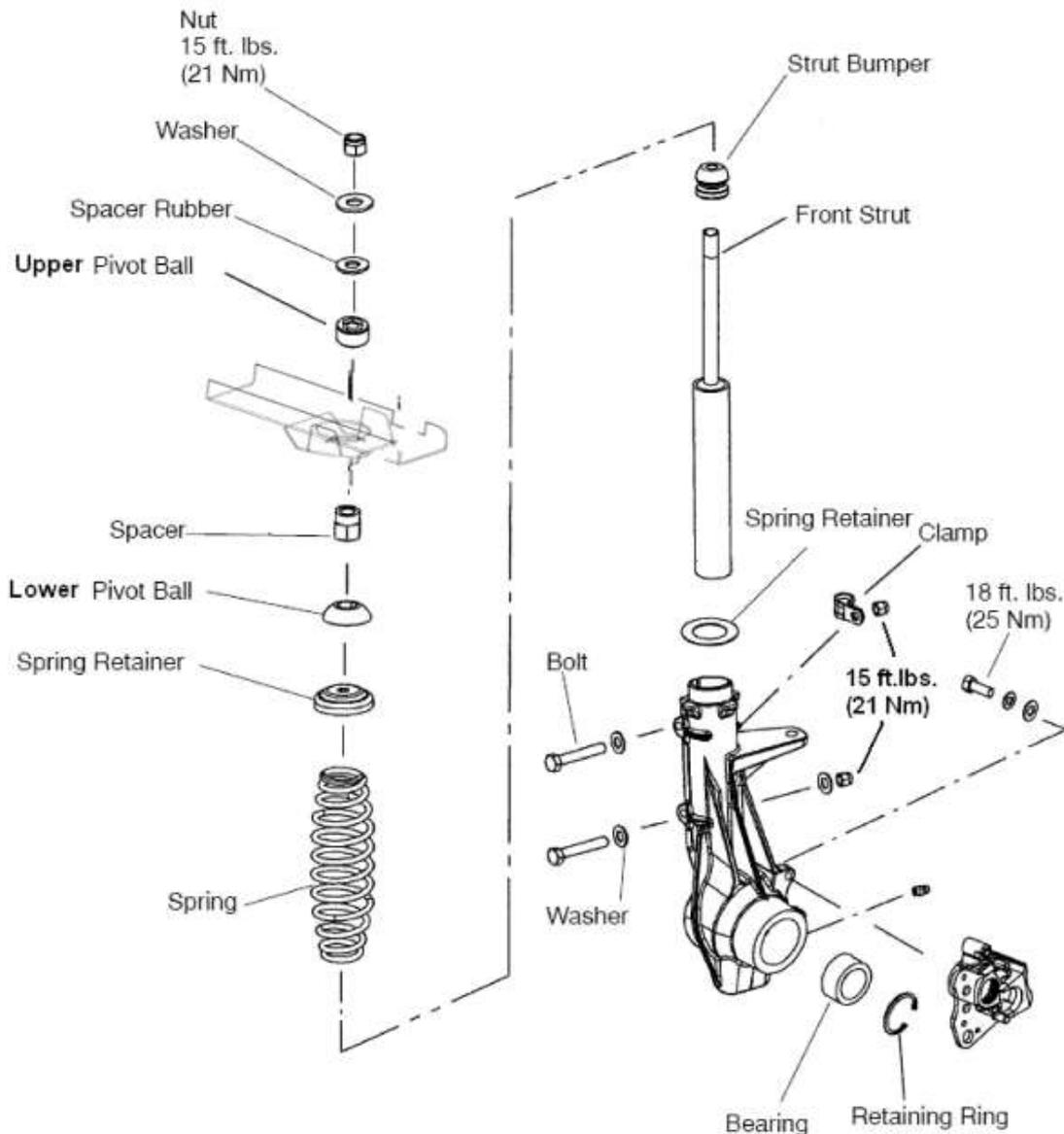
1. Hold strut rod with wrench and remove top nut.
