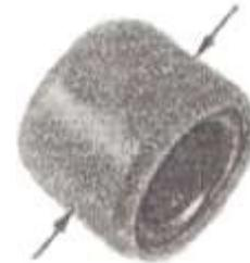
11. Measure sliding sheave inside diameter.
