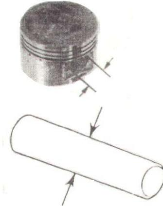
8. Measure piston outside diameter from an angle of 90° to piston pin bore, in a position some 9mm from piston bottom.
