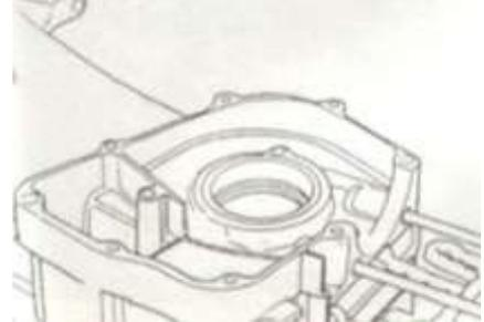
7. Remove oil seal from crankcase. Inspect oil seal for wear.
