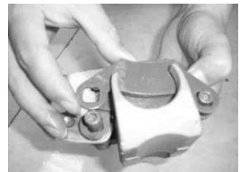
4. Slowly pump the brake lever until pressure has been built up. Maintain at least 1/2 "(13 mm) of brake fluid in the reservoir to prevent air from entering the brake system.
