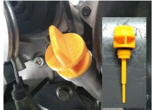
5. When replacing the oil, perform the first two steps and remove the oil strainer to drain the oil.
