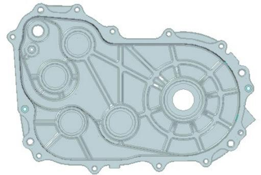
7. Prior to reinstalling the transmission make sure the mating surfaces are clean and dry, and shafts are fully seated in transmission case. Apply silicon glue to mating surfaces.
