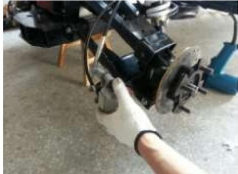
3. Remove the hub cap, cotter pin, spindle bolt, and washer.
