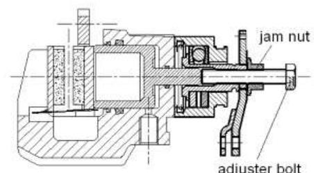
4. Tighten the nuts securely against the adjusters.
