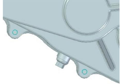
2. Remove transmission case fixing bolts.
