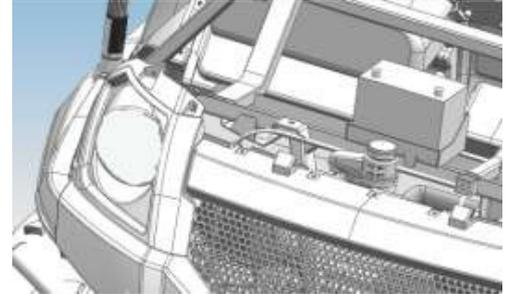
3. If changing fluid, remove old fluid from reservoir with a brake fluid pump or similar tool.
