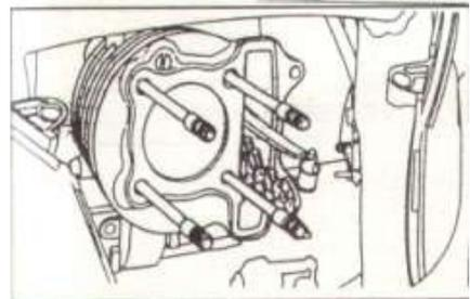
5. Remove dowel pin, cylinder head gasket and take out chain guide.
