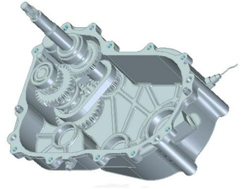
6. Remove the spindle assembly and countershaft assembly etc.
